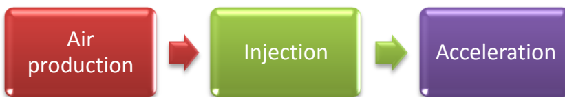
Function of multi-step micro-bubble aeration system
